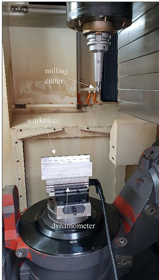
Figure 2. Measurement of cutting force components
